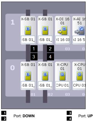
Figure 5-27: Connection of the System Bus
