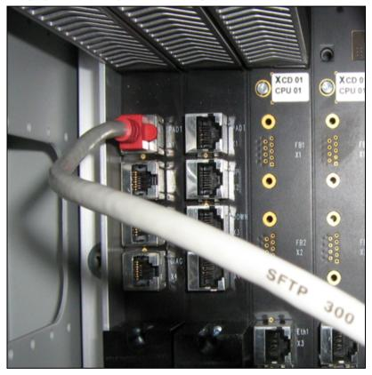
Figure 5-6: Connecting Ethernet Cables
