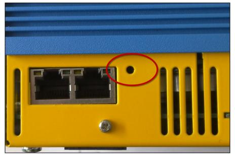
Figure 5-37: Reset Pushbutton
