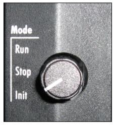
Figure 5-5: Mode Switch in INIT Position
