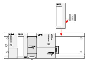
Repeat this procedure with the peripheral modules, by clicking a backplane bus coupler, stick the module right from the modules you've already fixed, click it downwards and connect it with the backplane bus coupler of the last module and bolt it.
