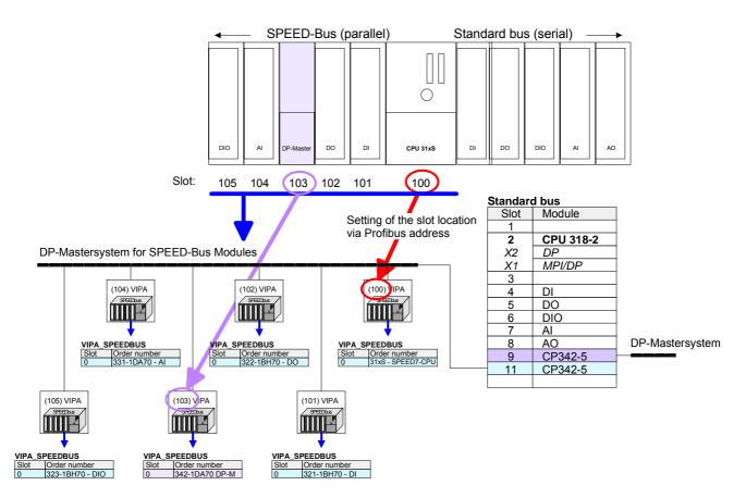
The according module is to be taken over from the HW Catalog of VIPA\_SPEEDBUS to slot 0.
