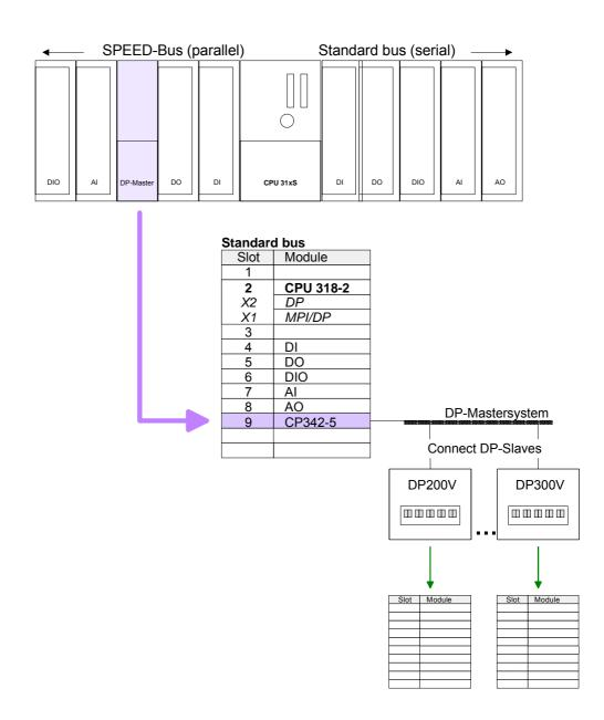
Project engineering of all SPEED-Bus modules in a virtual master system
