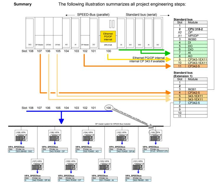
The according module is to be taken over from the HW catalog of vipa\_speedbus on slot 0.
