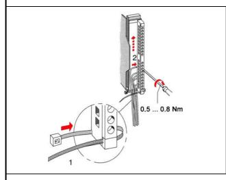
Put the included cable binder around the cable bundle and the front connector.
