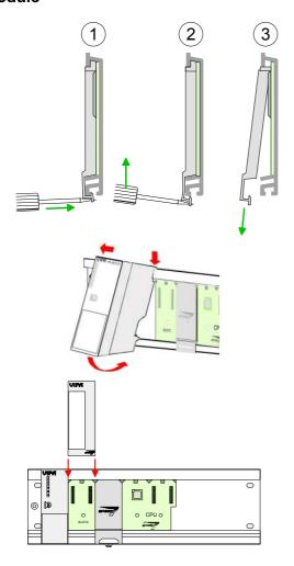
Dismantle the according protection flaps of the SPEED-Bus plug-in locations with a screw driver (open and pull down).
