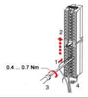
Fix the cable binder for the cable bundle.
