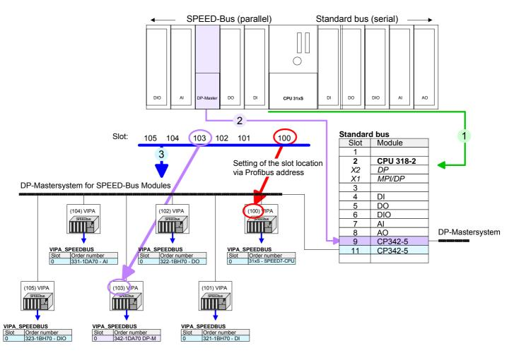
The according module is to be taken over from the HW Catalog of VIPA\_SPEEDBUS to slot 0.
