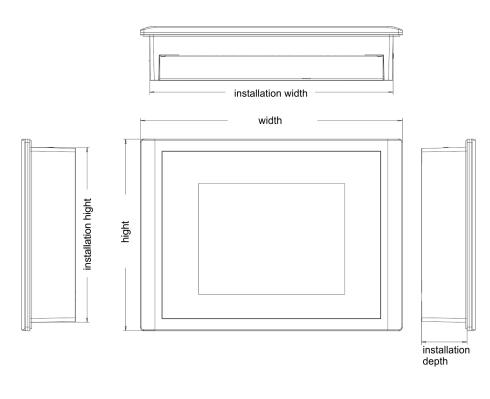
**Installation dimensions** For the installation of the Touch Panel in control cabinets and desks the following dimensions are necessary:
