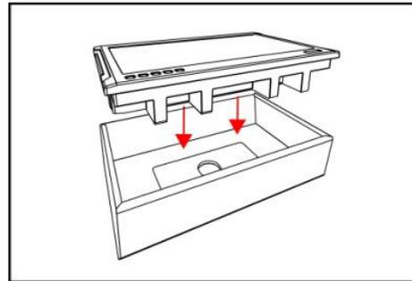
4. Mount the unit with a screwdriver (Tx10) on the surrounding housing. Use them to the provided screws (M3x8) and pull them by hand. Note the order of the gland.
