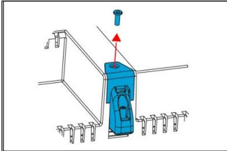
2. Screw the provided threaded bolt (M3x30 I / O) by hand in each Quick-Snap clamping bolt.
