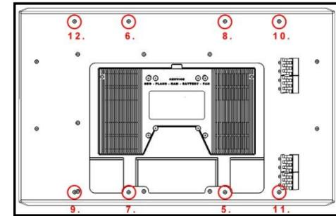
5. The VESA mounting holes are delivered with disc plugs. Before using the VESA mounting option, this must be removed accordingly. Unused VESA holes are to be kept closed with ribbed insert.
